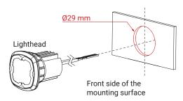
**NOTE:** To install more efficiently, use a rotating motion to guide the LIGHTHEAD when installing onto the cut-out.
