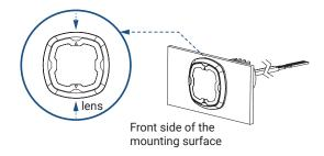
NOTE: Optical stripes must align vertically to meet regulation.
