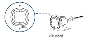
**NOTE:** Optical stripes must align vertically to meet regulation.
