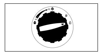
**Important:** Always ensure that the EZ Start dial and fuel lever vent are in the "OFF" position when the generator is not in use.
