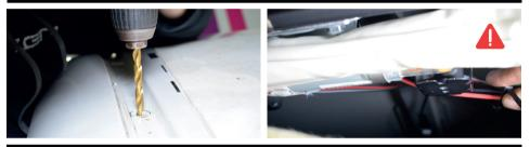
4. Depending on the light that is being installed and harness kit supplied, prepare the harness to allow you to feed the cable through the pre-drilled cable hole and cable grommet supplied.
