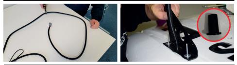
6. Add the rivets and using a rivet gun secure the bracket to the roof. Repeat step for right-hand side (minus cable entry).
