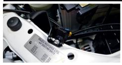
For vehicles that do not produce a constant 12v signal from the back of the headlight will require a CanM8 High Beam interface to control the signals. Please see our youtube channel, or scan the QR code for more infomation regarding install of the CanM8 interface.
