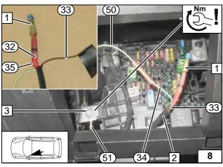
Connect red (rt) wire 32 and red/black (rt/sw) wire 35 according to wiring diagram.
